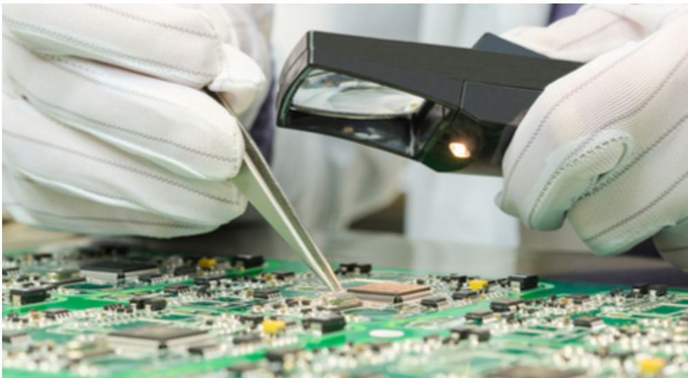
Inspecting the quality of soldered components on a PCB.
